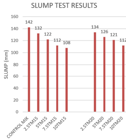
Fig. 1. Slump values obtained for different mixes.
