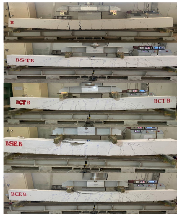
Fig. 6. Crack Pattern at the failure of tested specimens.
