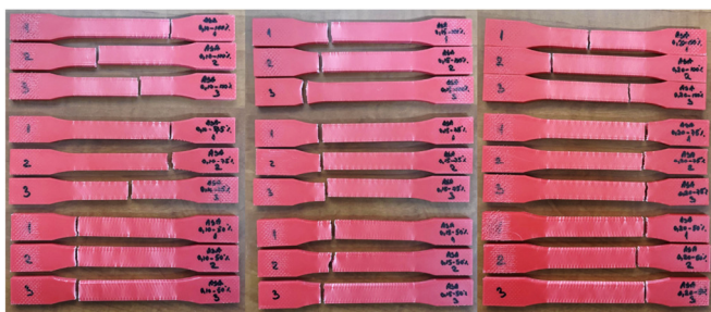
Fig. 6. ASA specimens after the tensile test.
