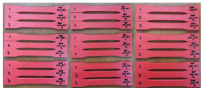
Fig. 4. ASA tensile test specimens manufactured by FDM on the Anycubic 4 Max Pro 2.0 printer.
