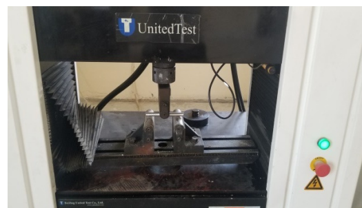
Fig. 6. Three point bending test.
