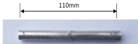
Fig. 3. Standard bending test specimen after welding.
