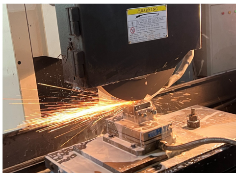
Fig. 2. Hardox 500 steel flat grinding experiment.
