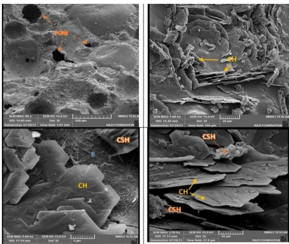
Fig. 8. SEM micrograph of the control mix.
