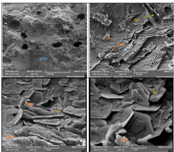
Fig. 9. SEM Micrograph of the mortar mix with marble powder.
