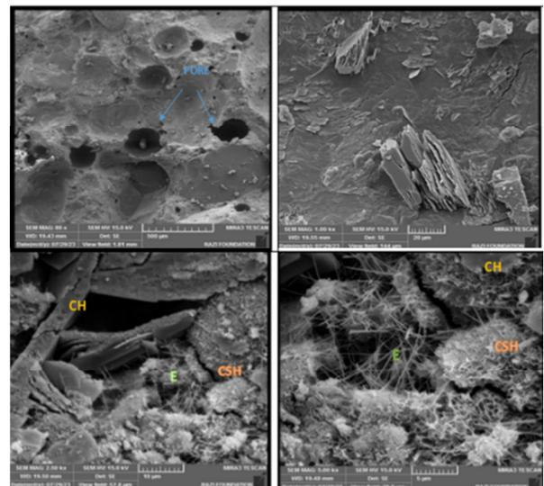
Fig. 11. SEM micrograph for mortar mix with porcelain+marble powder.
