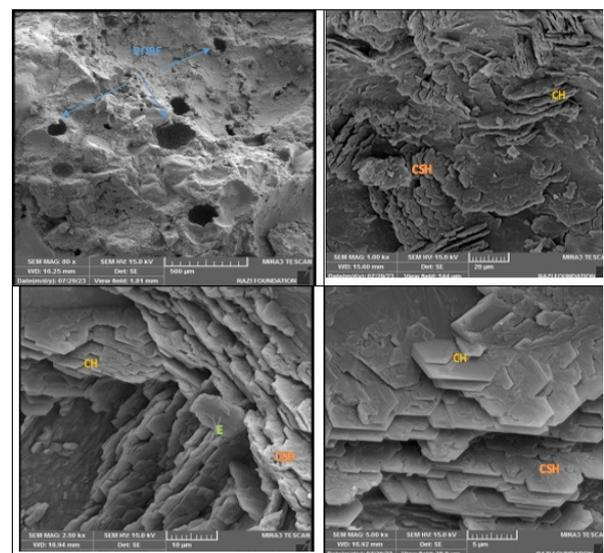
Fig. 10. SEM micrograph of mortar mix with porcelain powder.
