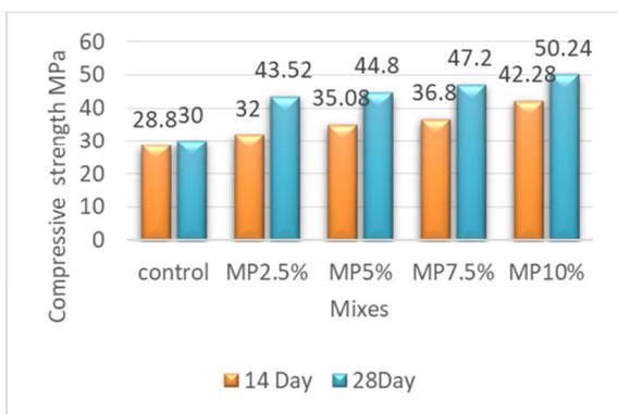
Fig. 6. Results of compressive strength test of M+ P mixtures at 14 and 28 days.
