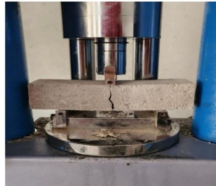
Fig. 3. Flexural strength test.
