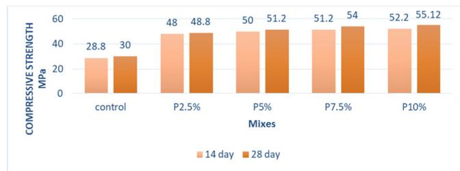
Fig. 5. Results of compressive strength test of P mixtures at 14 and 28 days.
