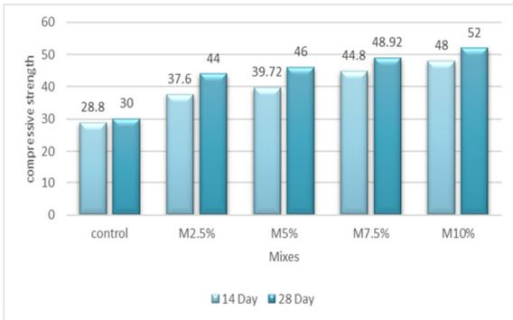
Fig. 4. Results of compressive strength test of M mixtures at 14 and 28 days.
