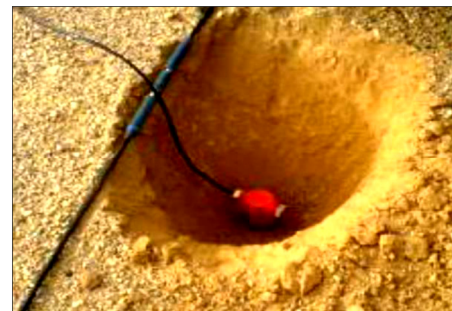
Fig. 6. A 40 HZ geophone layout in which a small hole is dug for better coupling.
