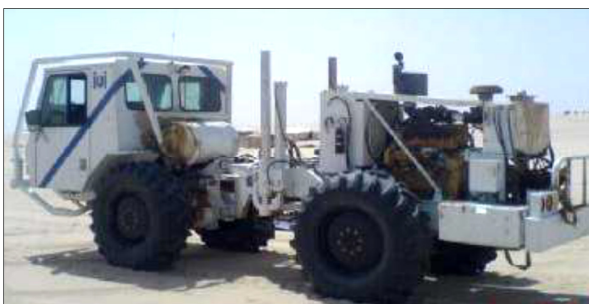
Fig. 5. Vibroseis used in the survey as the seismic source.
