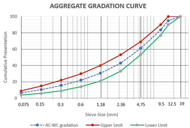
Fig. 3. Aggregate Gradation Curve for AC-WC.
