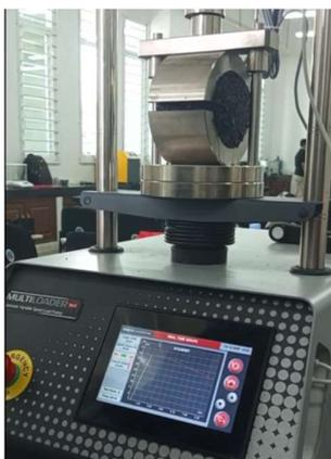
Fig. 4. Testing of DBE specimens using a Marshall Multiloader.
