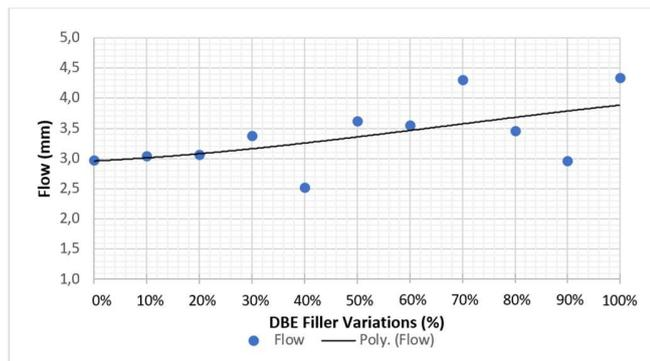
Fig. 9. Flow of the mixture with increasing DBE content.
