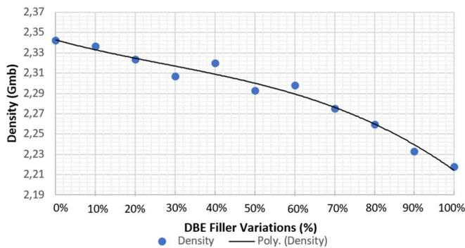
Fig. 5. Density of the mixture with increasing DBE content.
