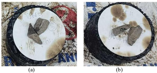
Fig. 6. (a) Oil spots on 80% DBE, (b) oil spots on 100% DBE.
