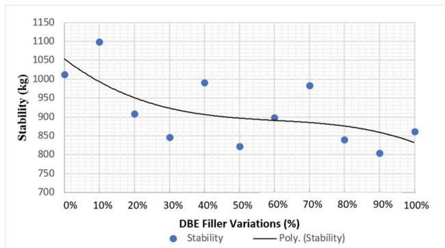
Fig. 8. Stability of the mixture with increasing DBE content.
