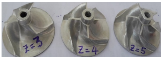
Fig. 4. Compressor wheels machined from CNC machines.
