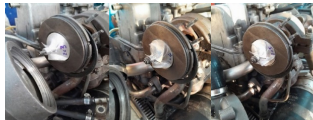
Fig. 6. The installation of compressor wheels in the turbocharger.
