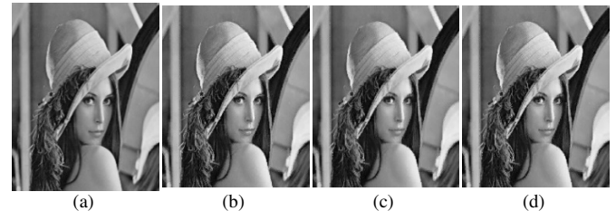
Fig. 6. (a) Original image, (b) Compressed image using MPBTC at CR=8, (c) Compressed image using AMBTC at CR=8, (d) Compressed image using EBTC at CR=8.
