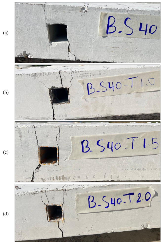
Fig. 6. Specimens failing at vertical openings (bottom view): (a) B-S40, (b) B-S40-T1.0, (c) B-S40-T1.5, (d) B-S40-T2.
