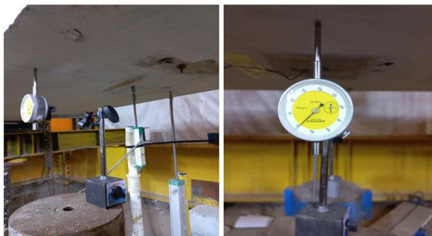
Fig. 6. LVDT and dial gauge test setup.
