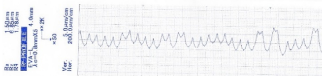
Fig. 11. Roughness profile of C40 Carbon steel with CT at 1300 rpm ( v_c = 36 m/min), a_p = 0.15 mm, f = 0.1 mm/rev.
