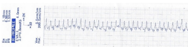
Fig. 12. Roughness profile of 201 stainless steel with UAT at 550 rpm ( v_c = 15 m/min), a_p = 0.15 mm, f = 0.1 mm/rev.
