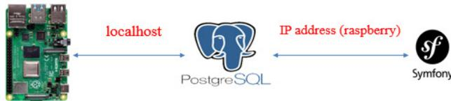
Fig. 5. Communication pipeline: integration of Symphony 6 and Raspberry Pi 4 with PostgreSQL for efficient data flow in Web development.
