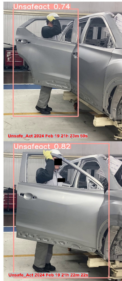
Fig. 4. Visual results of unsafe acts proof of concept of the proposed system.
