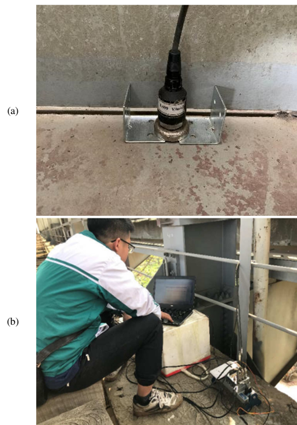
Fig. 4. Field data collection: (a) sensor installation, (b). control of the measurement process.
