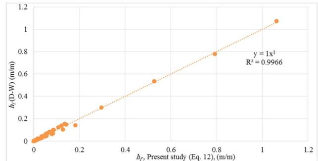
Fig. 2. Friction head losses by D-W against (12).
