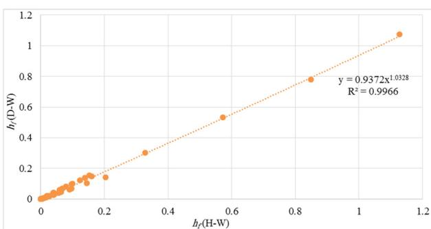
Fig. 1. Friction head losses by D-W against H-W.
