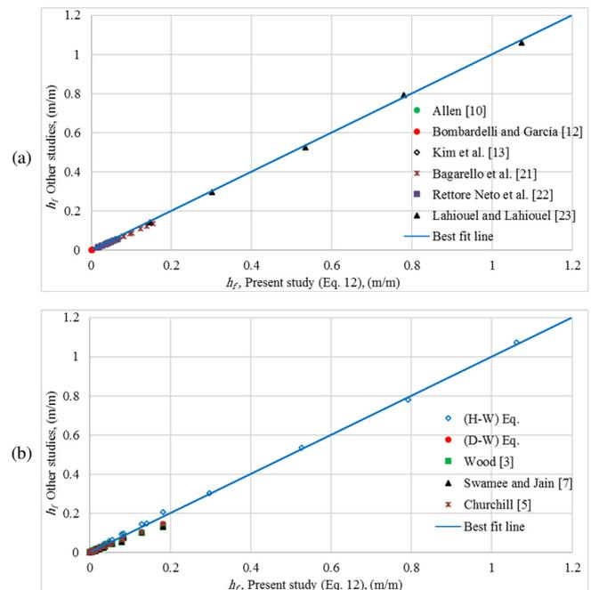
Fig. 3. Comparison between the friction head loss by (12) and: (a) experimental studies, and (b) numerical studies.
