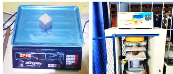
Fig. 4. Process of weighing samples and testing compressive strength.
