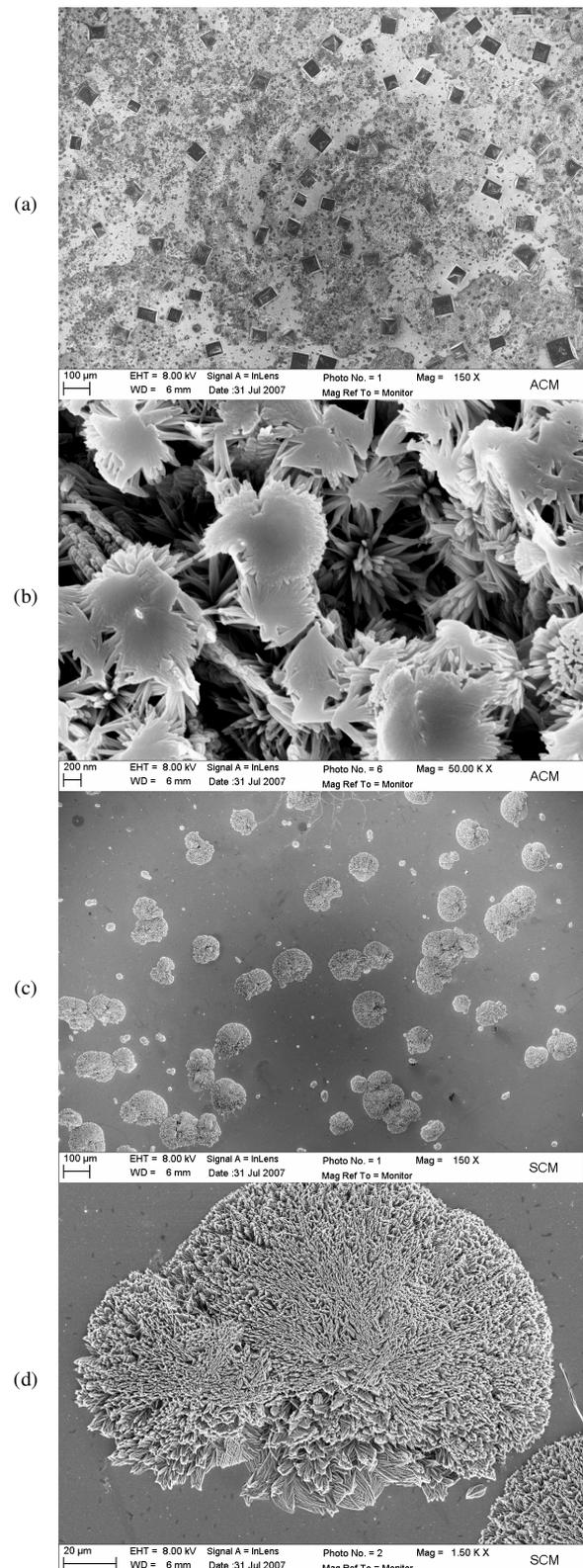
Fig. 5. SEM pictures of the solid surface: (a) with magnetic treatment, two layers, (b) with magnetic treatment, the first layer deposited, (c) without magnetic treatment, magnification 1, (d) without magnetic treatment, magnification 2.
