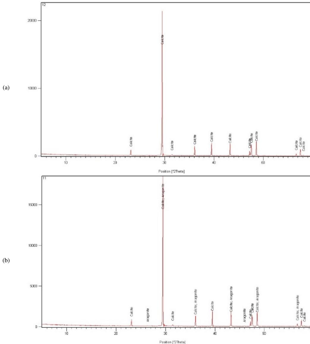
Fig. 6. XRD spectra of  $\text{CaCO}_3$  formed (a) without magnetic treatment and (b) with magnetic treatment.
