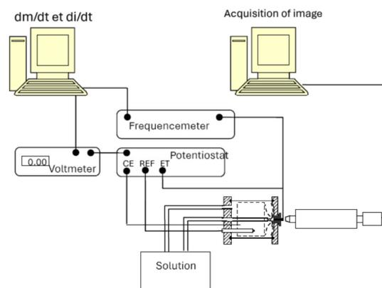
Fig. 2. Experimental setup of the electrochemical tests.
