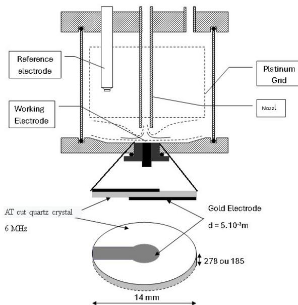
Fig. 3. Cell jet and working electrode.
