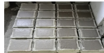
Fig. 2. Casting of PQC cubes.
