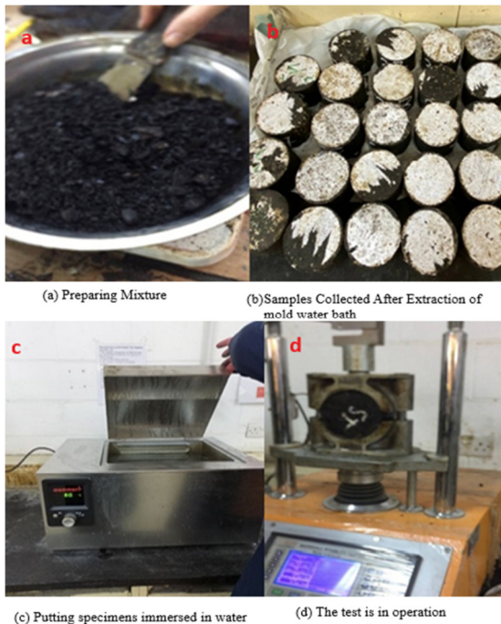
Fig. 3. Testing of Marshall specimens.
