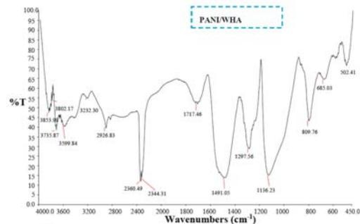
Fig. 3. IR spectrum of WHA Nano-composite/poly-aniline
