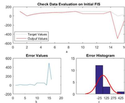
Fig. 8. Difference between ANFIS output and detailed output during the testing stage
