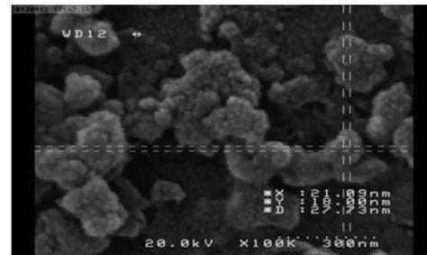
Fig. 2. SEM image of WHA Nano-composite/poly-aniline
