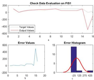
Fig. 10. Difference between ANFIS output and detailed output during the testing stage of FIS1
