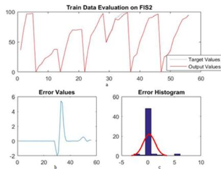
Fig. 11. Difference between ANFIS output and detailed output during the training stage of FIS2
