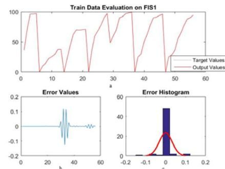
Fig. 15. Difference between ANFIS output and detailed output during the training stage of FIS1
