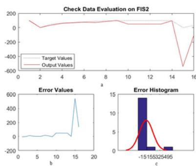
Fig. 18. Difference between ANFIS output and detailed output during the testing stage of FIS2
