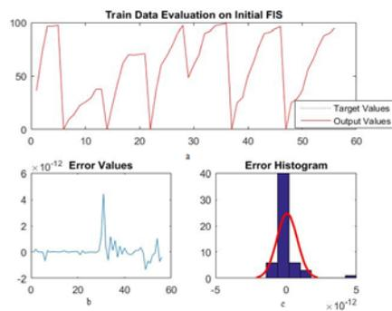
Fig. 13. Difference between ANFIS output and detailed output during the training stage of FIS
