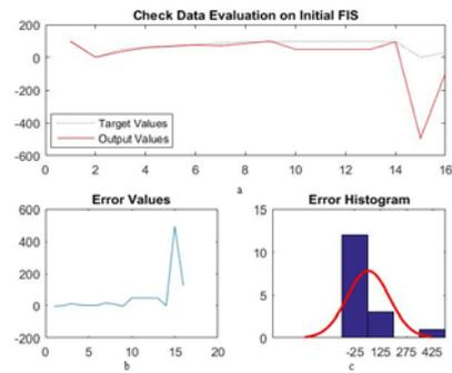
Fig. 14. Difference between ANFIS output and detailed output during the testing stage of FIS
