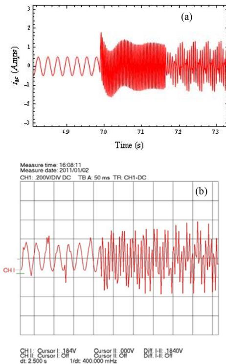
Fig. 4. Current responses of cases 1 and 2: (a) simulation, (b) experimental
