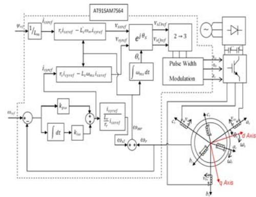
Fig. 1. Rotor field oriented vector control drive.
