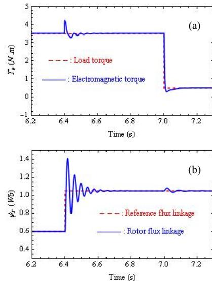
Fig. 3. Vector control response: (a) Flux linkage response, (b) Torque response
