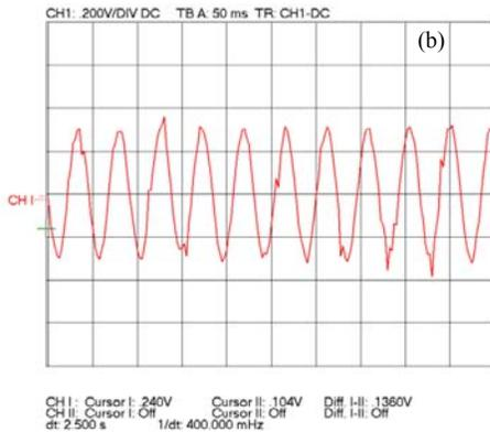
Fig. 8. Current responses for case 3: (a) simulation (b) experimental
