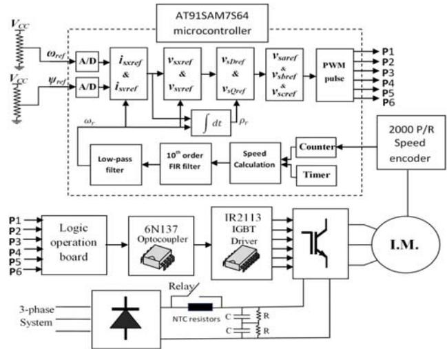
Fig. 2. Experimental set-up diagram.
