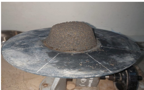
Fig. 3. Flow table test of RHA-CBA mortar.
