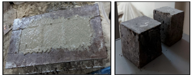
Fig. 4. Mortar specimens during casting and before testing.
