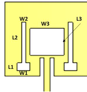
Fig. 1. Geometrical representation of the hammer-slotted patch antenna.
