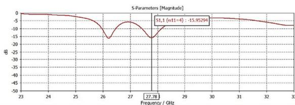
Fig. 2. S11 as a function of frequency for the proposed antenna.
