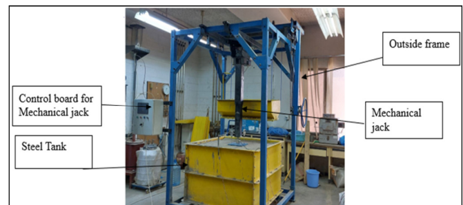
Fig. 1. Steel tank model with a mechanical jack.
