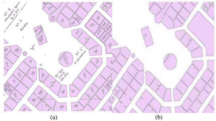
Fig. 5. Extracted features in a vector format: (a) The initial features with labels, (b) results from label removal through a feature merge operation. The labels inside the polygons were removed significantly.
