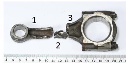
Fig. 3. The connecting rod is broken into 3 pieces.
