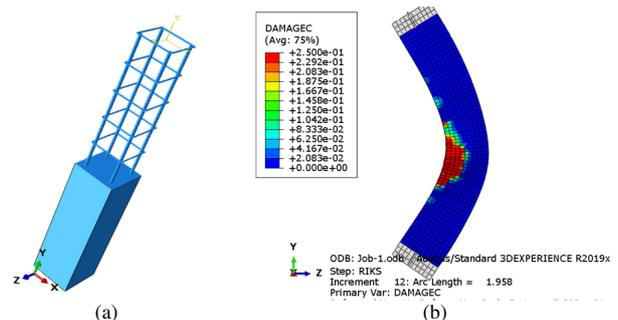
Fig. 1. Model 1: (a) view cut, (b) failure mode.
