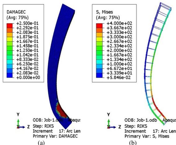
Fig. 11. Model 5: (a) failure mode, (b): reinforcement stresses.
