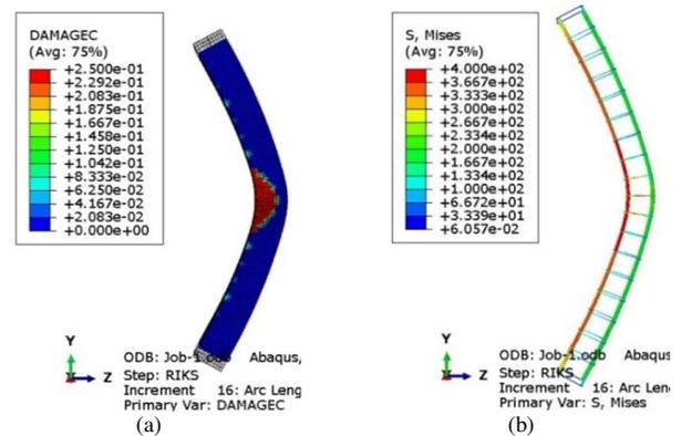
Fig. 4. Model 2: (a) failure mode (b) reinforcement stresses.
