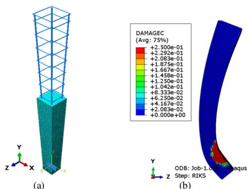
Fig. 7. (a) View cut of meshed Model 3, (b) Failure mode of Model 3.
