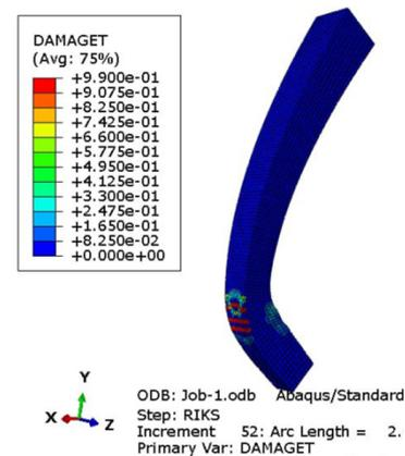
Fig. 12. Tensile cracks in Model 5.
