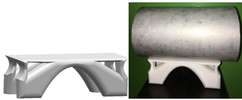
Fig. 12. The completed prototype received a 59% decrease in weight.
