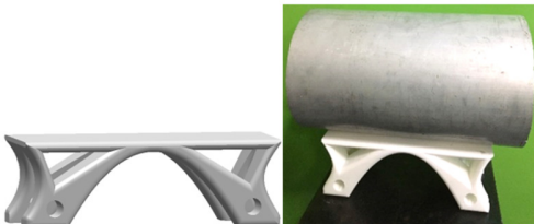
Fig. 13. The completed model received a 70% decrease in weight.
