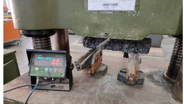
Fig. 4. Prism specimen under flexural strength test.
