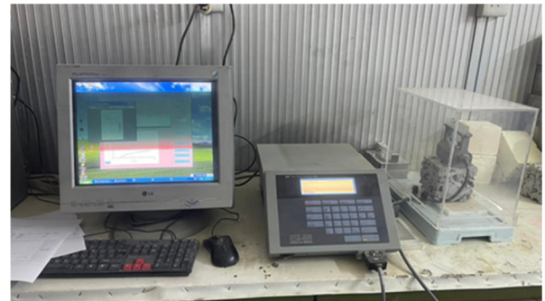
Fig. 5. Cube specimen under thermal conductivity test.
