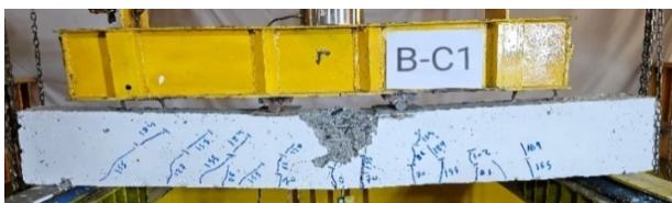
Fig. 12. Mode of failure of B-C1 beam.
