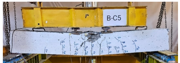
Fig. 16. Mode of failure of beam B-C5.
