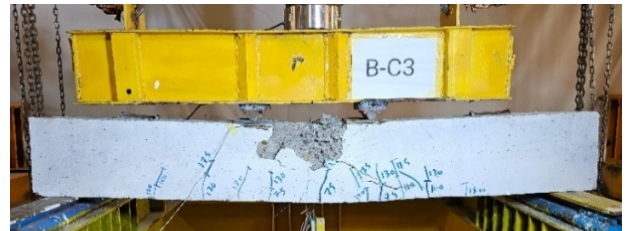
Fig. 14. Mode of failure of B-C3 beam.
