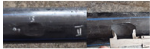
Fig. 3. Pipe with defect (Pipe II).
