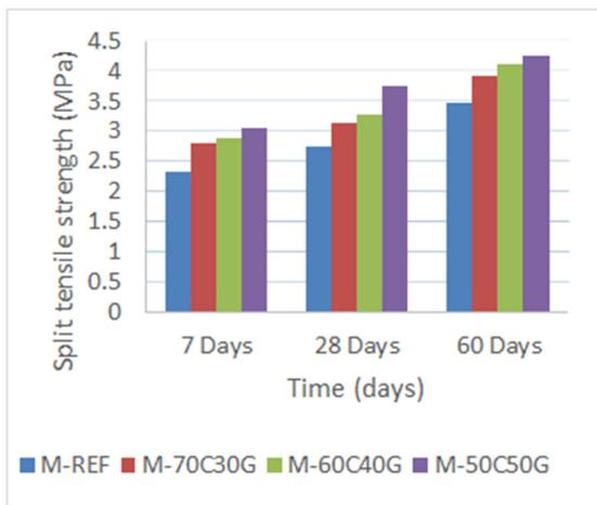
Fig. 7. Split tensile strength test result.
