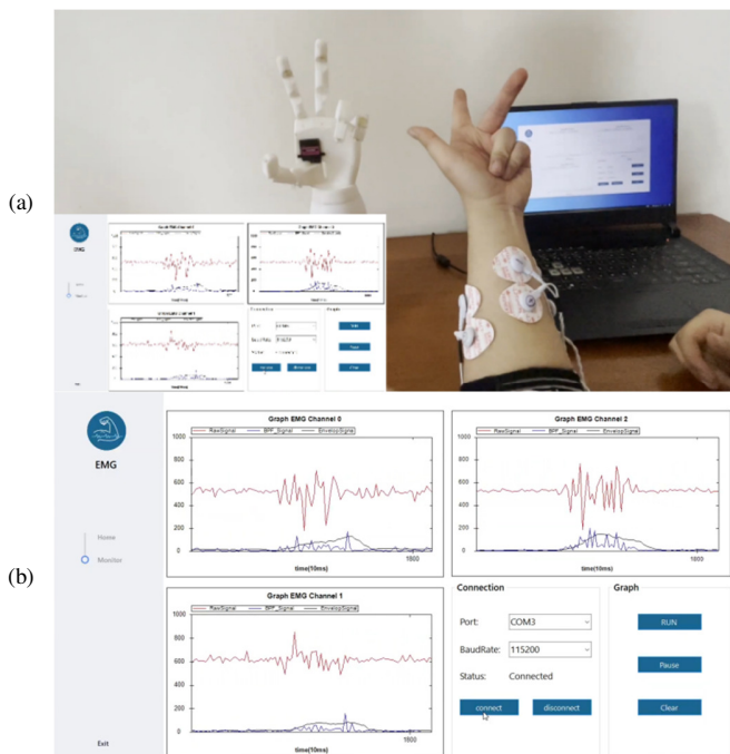
Fig. 8. Experimental results on the robotic arm model applied sEMG signals - controlling the pinky and ring fingers: (a) curl the fingers and (b) waveform graphs.
