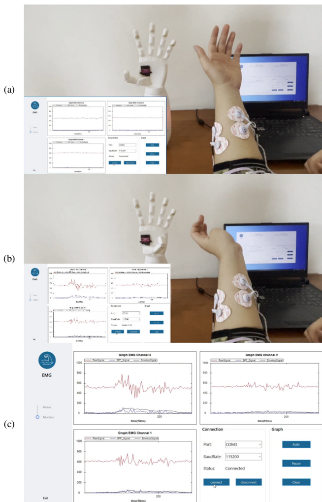
Fig. 6. The experimental results on the robotic arm model applied sEMG signals - thumb control: (a) Relax the hand, (b) Curl the thumb, and (c) waveform graphs.
