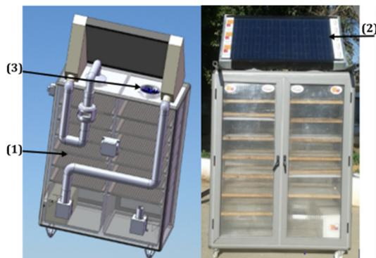
Fig. 1. Experimental solar test bench of the dryer with PVT.
