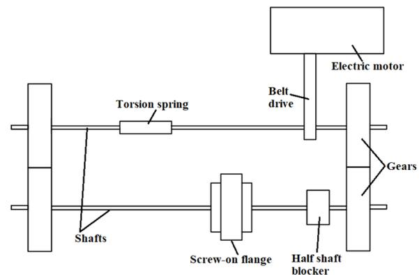
Fig. 1. Schematic representation of the wear testing equipment.
