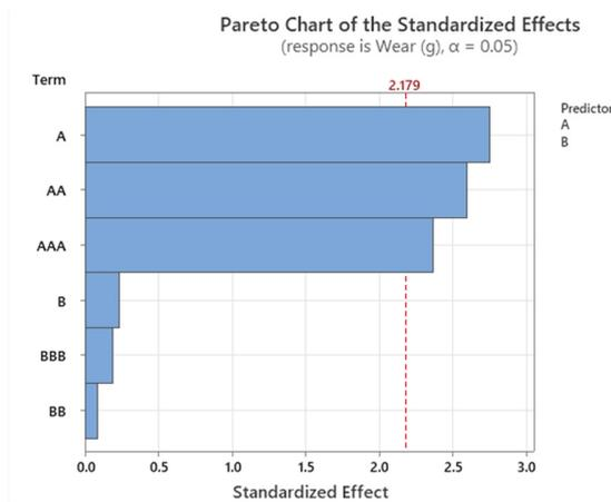
Fig. 5. Example of Pareto chart used to establish the significance of terms used for regression analysis (PLA annealed).
