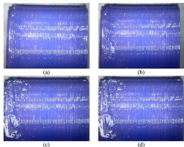
Fig. 7. Wear images of the flank of the teeth: (a) at the beginning, (b) after 30 min, (c) after 60 min, (d) after 120 min.
