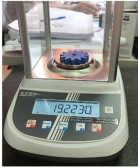
Fig. 2. Analytical balance used to determine the mass of spur gears.
