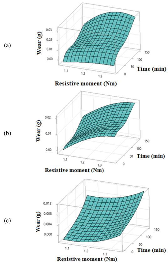
Fig. 6. Wear variation against torque and time: (a) PLA gears, (b) annealed PLA gears, (c) ABS gears.
