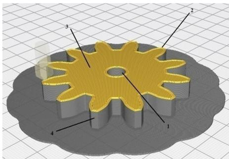
Fig. 4. Sliced gear model: 1-specimen; 2-shells; 3-infill pattern; 4-overlapping layers.
