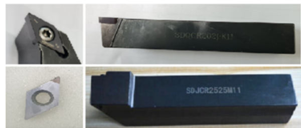
Fig. 2. Carbide cutting tool for turning 9XC alloy steel.
