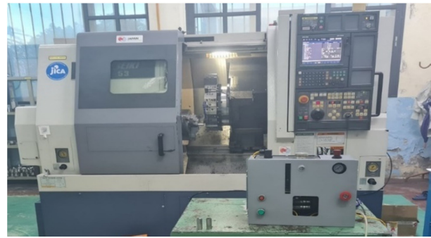
Fig. 3. MQL-assisted CNC lathe experimental setup.
