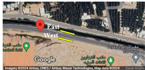
Fig. 3. Location of the Spot Speed Study (25°23'37.5"N, 49 49°39'09.0"E) in East-West direction. Trap length: 110 m (Map data: Imagery@2024, Airbus,CNES/Airbus, Maxar Technologies).
