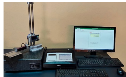
Fig. 4. Calibrated Mitutoyo surface roughness tester model SJ-310.
