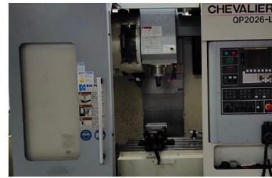
Fig. 1. The CNC milling machine (3axis).
