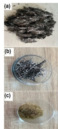
Fig. 1. Fibers used in RPC reinforcement: (a) CF, (b)WSF, (c) MSF.
