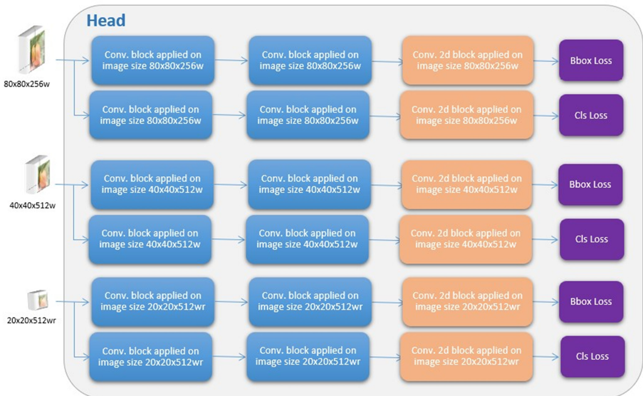
Fig. 8. The structure of the head block.
