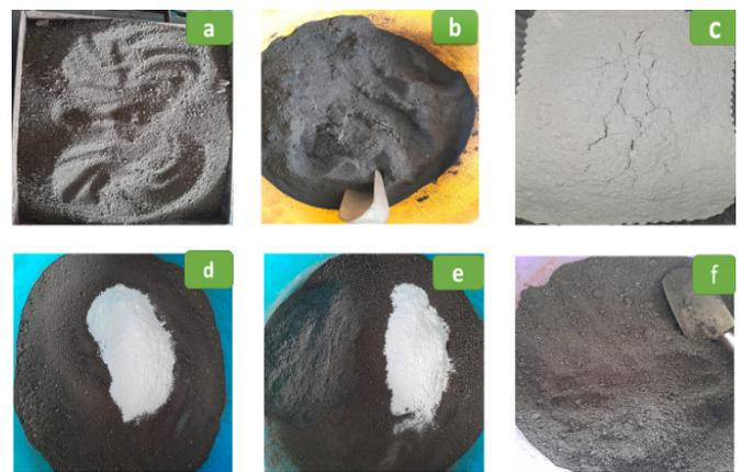
Fig. 1. (a) Expansive soil, (b) CCA, (c) WMD, (d) soil mixed with WMD, (e) soil mixed with CCA, (f) Soil mixed with WMD and CCA.
