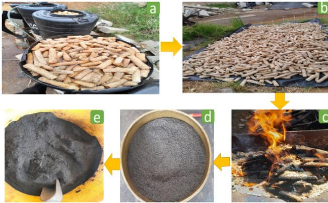
Fig. 2. Treatment and preparation of CCA: (a) Soaking of cobs, (b) drying of cobs, (c) incineration, (d) sieving, (e) ash.
