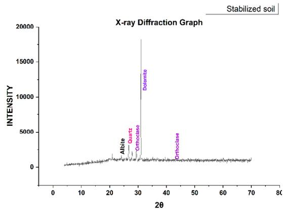
Fig. 14. XRD analysis of stabilized soil.
