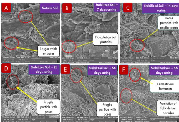
Fig. 12. SEM images for 7 - 90 days of curing.
