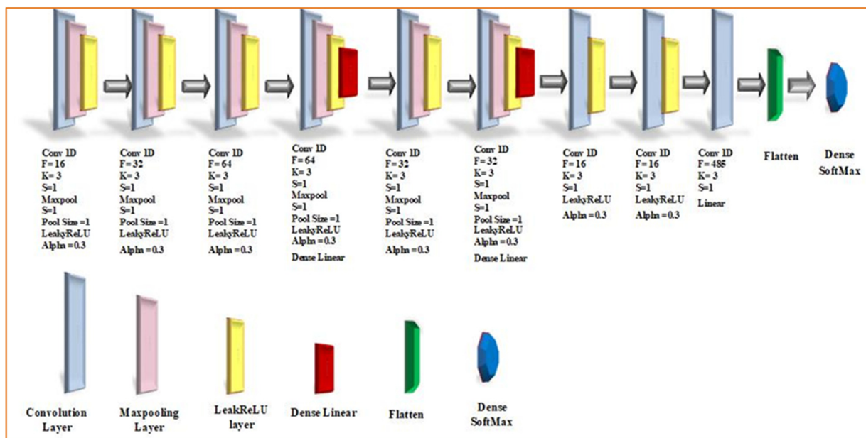
Fig. 7. Architecture layers of the proposed 1D-CNNHM.
