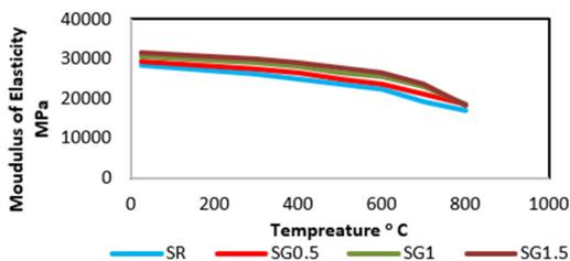
Fig. 7. Effect of burning temperature on the modulus of elasticity of SCC.
