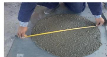
Fig. 3. Slump flow test.
