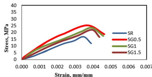
Fig. 13. Stress-strain at 600°C.
