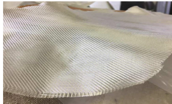
Fig. 2. Glass fabric used in the production of the test samples.
