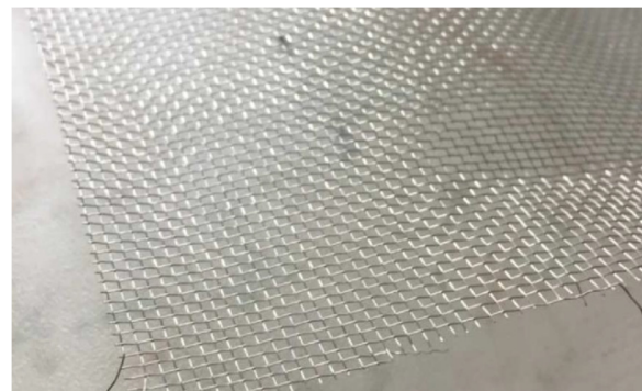
Fig. 4. Metal grid with a mesh size of 2 × 2 mm applied as a specific layer of D samples.
