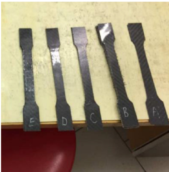
Fig. 6. Samples prepared for the tensile test.
