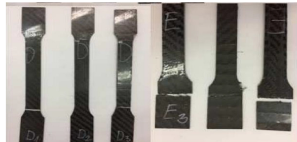
Fig. 7. Broken samples after the tensile test.
