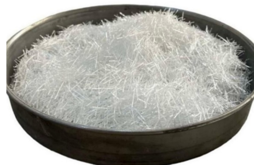
Fig. 1. PET fibers prepared in this study.
