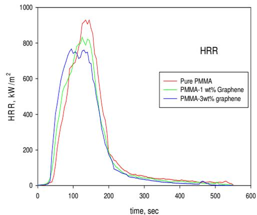
Fig. 4. Average heat release rate for pure PMMA and PMMA-graphene composites.
