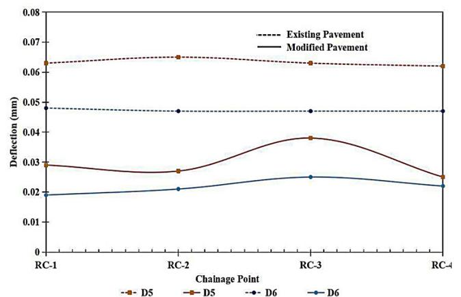
Fig. 6. Deflection variation in subgrade for both pavements.
