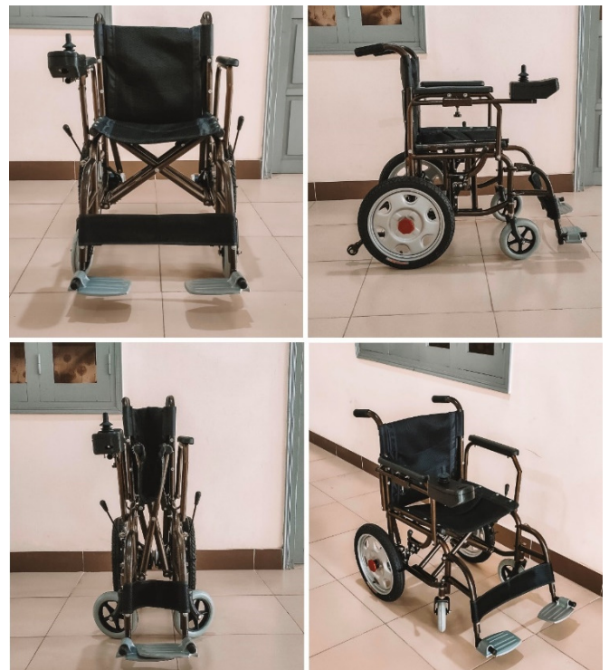
Fig. 6. A prototype of the electric wheelchair.
